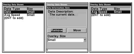
Overlay Data Shown, with Date option selected (left). Press ENT to access REMOVE option (center). Press ENT again to remove item and return to Overlay Data Shown (right).
